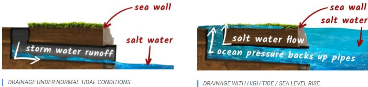
Figure 10: High Tide Flooding
